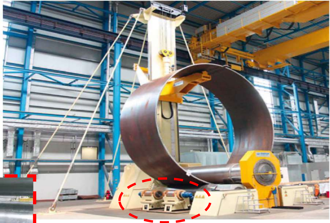
Handling system for pipe segments and cones. 搭配半圓成型或Cone錐體捲圓作業用
