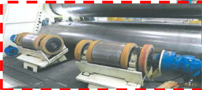
Handling system for pipe segments and cones. 搭配半圓成型或Cone錐體捲圓作業用
